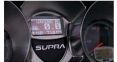
Integrated PerfectPass speed control system with one-touch control that remembers a rider's preferred speed setting and holds it to within 0.2 mph.
